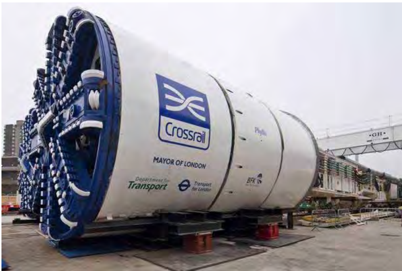
Big job: the TBMs used in boring weigh just shy of 1,000 tonnes
